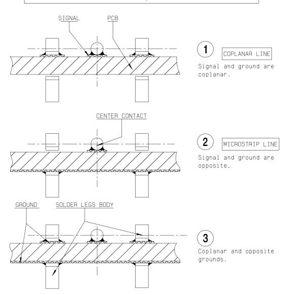
Solution (3) features a stronger mechanical retention on the PCB because the 4 leads are soldered.
